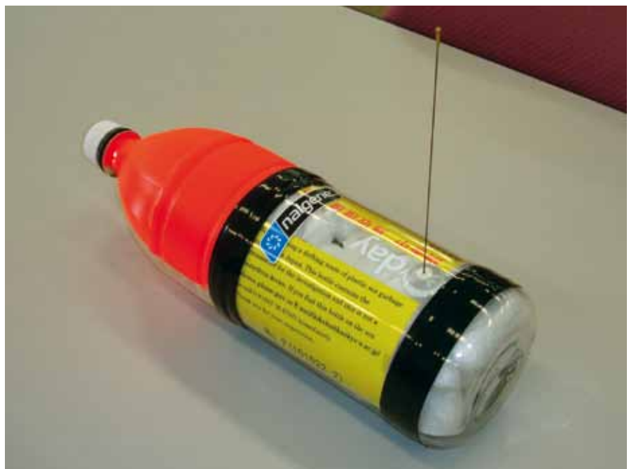
The Argos transmitter disguised as an ordinary plastic bottle was designed and developed by Nomad Science. The transmitters were deployed in the aftermath of the Great Earthquake and Tsunami.
